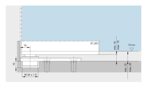
Using the bottom patch on pivot bearing with cover plate (Art. No. 01.201) the air gap between floor and glass is 15–20 mm (by height adjustability).
